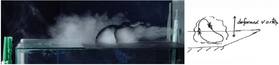
Fig. 15 Photograph showing three superimposed images of a smoke vortex ring colliding with a rigid plane surface. They show the smoke ring bending down towards a rigid floor, and lifting up again as a puff of smoke. A schematic of the vortex deformation as it interacts with the floor is shown on the right
