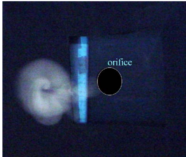
Fig. 13 Elevated view of a vortex ring, with net swirl, emitted from the vortex generator and visualised with smoke. The background image shows the vortex generator
