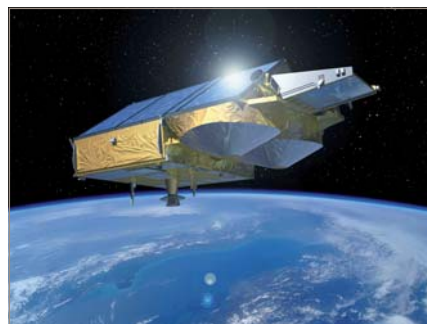
Fig. 2. Planned European CryoSat satellite (2008) for monitoring polar ice fields (ESA/P.Carril)
